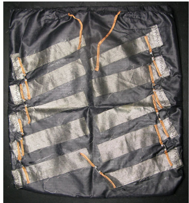
Fig. 4 Inside view of prototype skirt panel. 10 electrodes (each ~2.5 cm × 10 cm) were cut out of conductive organza and affixed to the nylon substrate using spray fabric adhesive. Diodes were soldered to sections of copper braid and sewn across the organza strips. Two additional sections of copper braid were sewn to the terminal electrodes to allow connection to external circuitry
